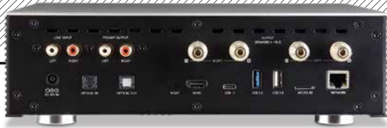
ABOVE: Line in/pre out (RCAs) are joined by optical digital in/outs and 4mm speaker cable terminals. There's an Ethernet port plus one USB-C, micro SD and two USB-A ports for external media and a BT/Wi-Fi dongle. Optional SSD is loaded under the case
